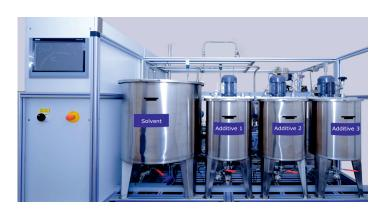
Eight different liquid feeds with versatile viscosities are dosed into three static mixers to deliver the end product mixture, which is then used further in the production process. The plant can produce different polymer concentration mixtures and the produced amount can be regulated based on the daily supply demand of the customer. The continuous mixing system is fully automated and can easily be connected to the local site IT system, such as SAP.
